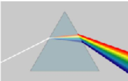
In a prism, material dispersion (a wavelength-dependent refractive index) causes different colors to refract at different angles, splitting white light into a rainbow.
