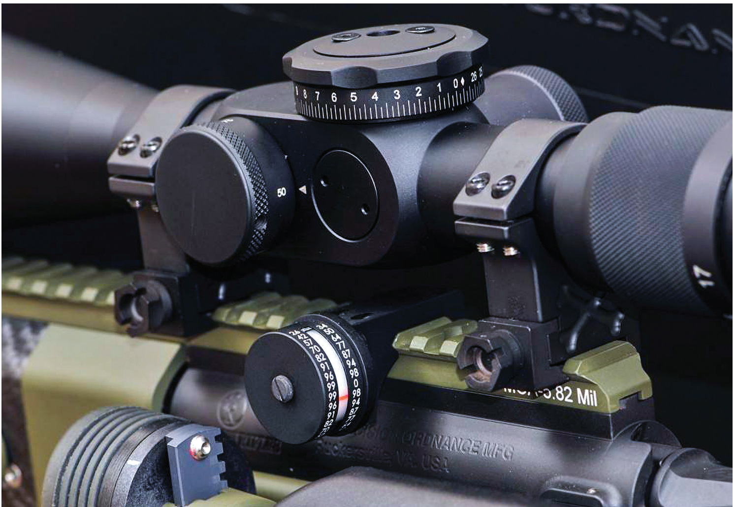
Sniper Tools Design Company's Angle Cosine Indicator—used by most military snipers under the NATO umbrella.
